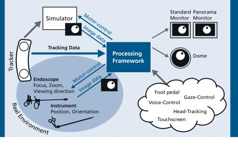
A highly efficient, componentbased software platform called »Endoguide Processing Framework« is the centerpiece of the endoscopic system
