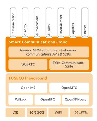
Using the NGNI FUSECO Playground, services and technologies for seamless communication can be tested close to reality
