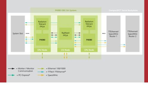
Embedding the P4080 system (DMR) to the OBC-SA connection structure
