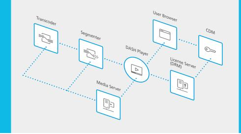
The FAMIUM DASH solution forms a end-to-end system from content creation to content consumption
