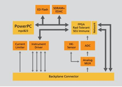
Functional Block Diagram of the TET-Control Computer
