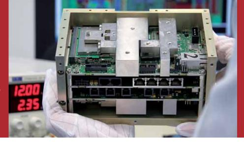
The eight processor cores of the P4080 are not only used to maximize computing power, but also for the realization of potent mechanisms for fault tolerance.
